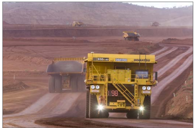
Figure 2 - An autonomous haul truck in operation at Rio Tinto's West Angeles mine site in western Australia. Image, courtesy Robe River Iron Associates.
