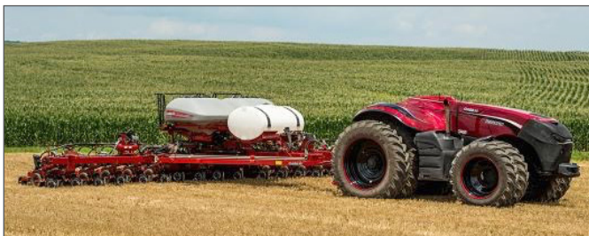
Figure 1 - CNH Industrial's concept autonomous tractor can perform a number of agricultural duties, including driving out to a particular field, performing a task, and driving back to the barn. Be sure to watch the video in the References Image, courtesy CNH Industrial.
