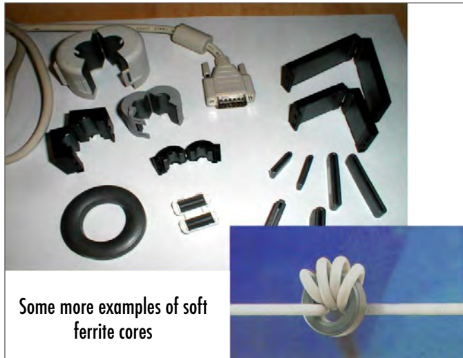
Figure 7 - Some more examples of soft ferrite cores
